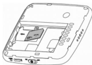
3. Insert 4G SIM Card with the Verizon Wireless logo facing you into the slot until it is fully inserted.
