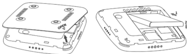
2. Place the battery cover over the battery compartment ensuring that the arrow on the device and the arrow on battery cover are aligned. Then press the battery cover downward until it clicks into place.
