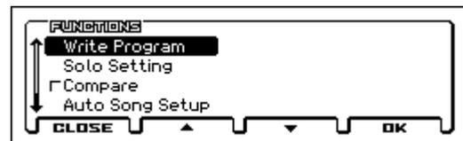
For example, suppose that you're in Program mode and press the FUNCTION button to access the function list.
