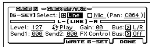
**Note:** It's not possible to input audio via both the LINE IN jack and MIC IN jack simultaneously.
