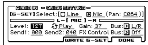
2. In the Select area, specify the input jack that you want to enable. Set the appropriate Level and Gain settings. (see "Connecting your input devices" on page 18)
