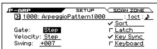
When specifying Gate, Velocity, and Swing, set the PROG> ARP page parameters [GATE], [VEL], and [SWING] to +00.
