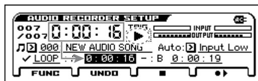
**Note:** If you use this method to specify the time location of a point, the location will be specified with an accuracy of within one second.
