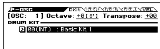
4. Specify the basic pitch of the oscillator. For a drum kit, set “Octave” to +0 [8’].
