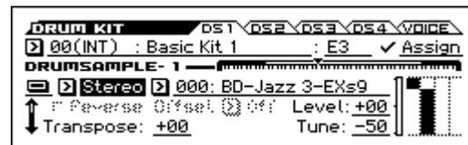
4. Select a drum sample. Select Drumsample 1, and press the ENTER button.
