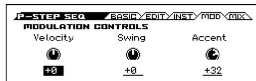
2. Velocity adjusts the basic volume, SWING adjusts the sense of swing, and Accent adjusts the volume.
