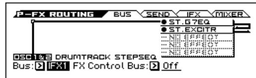
2. “Bus (Bus Select)” specifies the bus where the output from the oscillators will be sent. Here we’ll choose IFX1 so that the output of the oscillators will be sent to insert effect 1.
