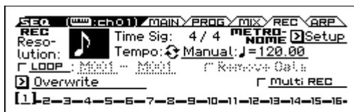
For example if REC Resolution is set to ♩, the timing of your realtime-recorded notes will be automatically adjusted as shown in section “2” of the following illustration whenever it varies from 8th note intervals.
