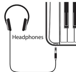
The KROSS's Headphone jack will output the same signal as the OUTPUT L/MONO and R jacks.
