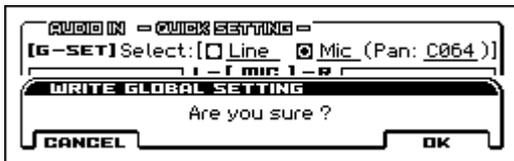
5. To save the settings, press the WRITE G-SET (PAGE+) button. A dialog box will appear; press the OK (MENU) button to save the settings.
