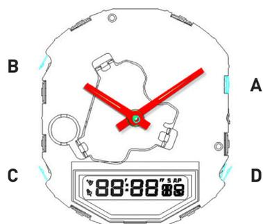
In any mode, press and hold Key A for 2 second to adjust the analog time.
